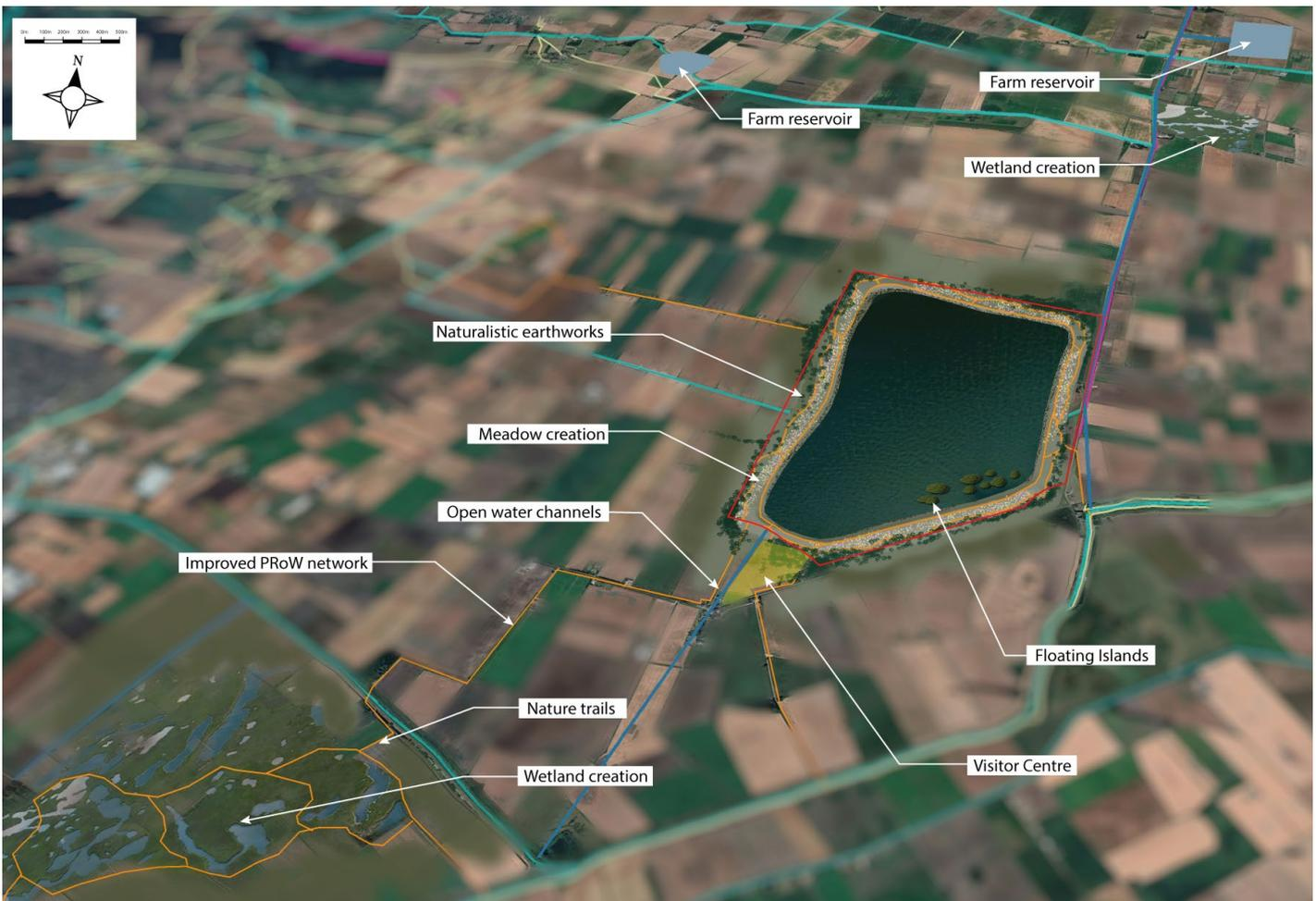
In addition to this, local sources would be captured and stored within two 0.5MCM bank storage wetlands to support water supply both for irrigation and the PWS reservoir. The design for these would be the same as for CDO2.
