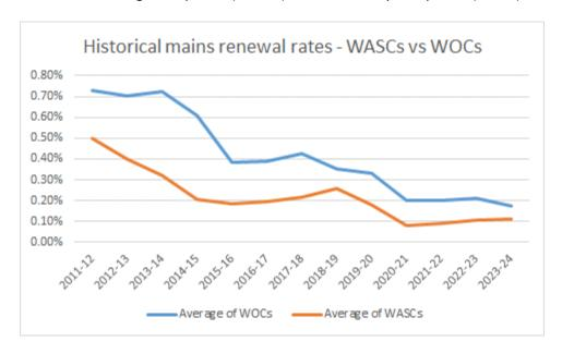
The industry level weighted mean over-predicts WASC lengths significantly (8,360km vs 7,384km) whereas under-predicts for WOCs (1,538km vs 2,567km). To remedy this, is it possible to produce weighted means for WASCs and WOCs separately, being respectively 0.21% per annum and 0.40% per annum. This effectively closes the gap between predicted and actual km (WASCs: 7,315km vs 7,384km, and WOCs: 2,564km vs 2,567km).
