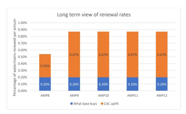
This Cost Adjustment Claim is to increase the level of capital maintenance within Anglian Water's allowance, to allow an increase in the mains renewal rate to 0.54% within base for AMP8 (2025-2030). We calculate the required increase in capital maintenance using our own cost models, which indicate a unit rate below Ofwat's efficient unit rate.
